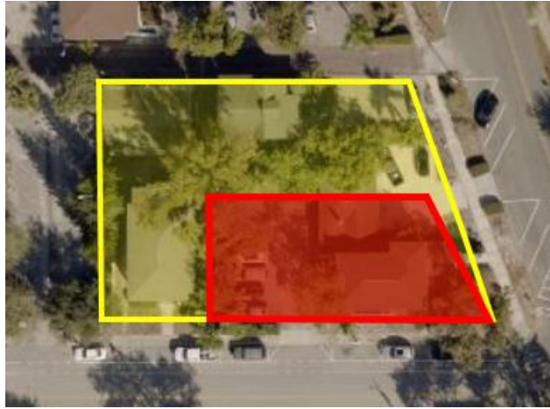
Figure 26. Footprint of 6-story portion of “The Mirror” [red] shown inside footprint of proposed base (pedestal) [yellow].
